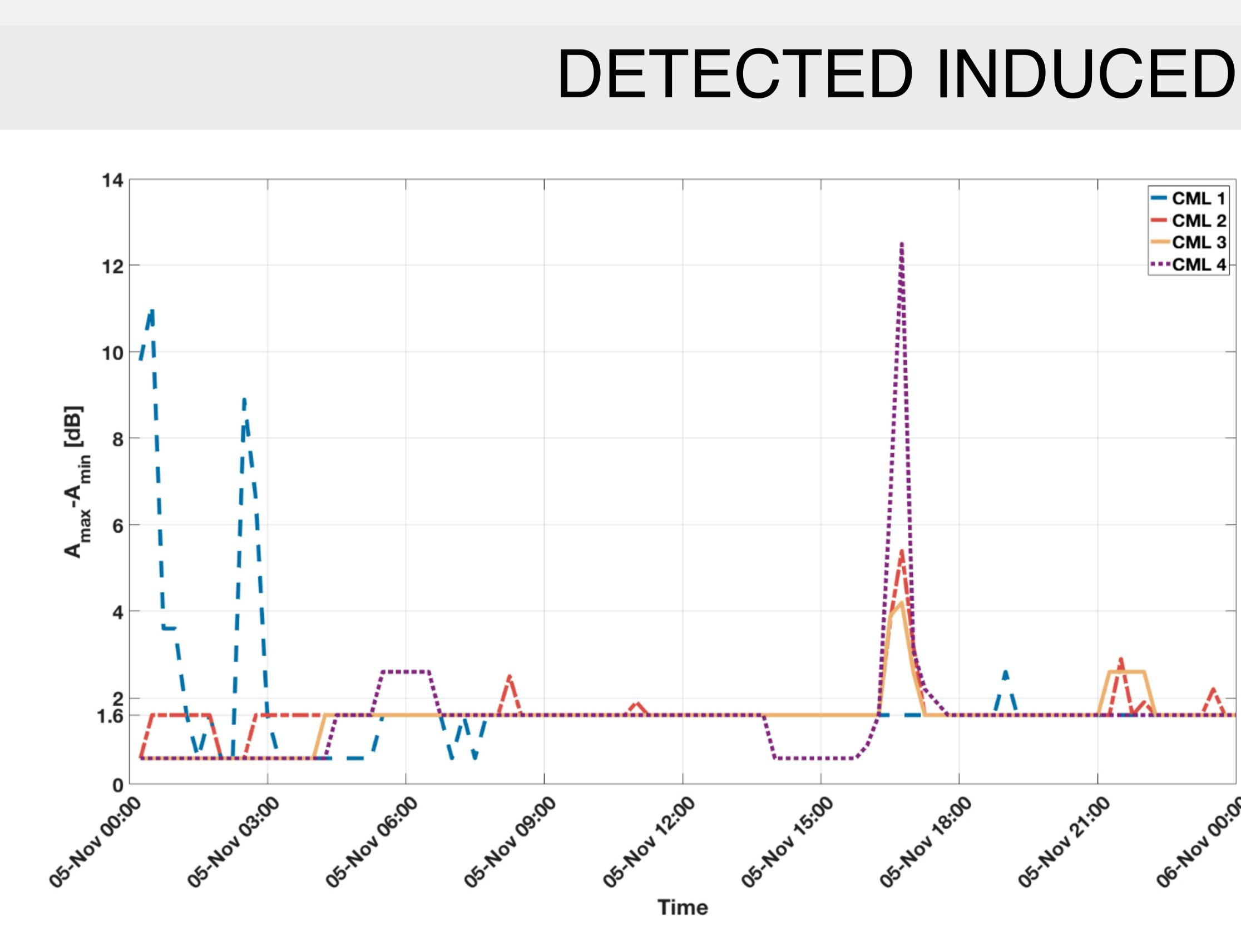
This paper deals with CMLs measurements which are produced by current NMS. We show that the measurements which are being produced by these systems include an inherited bias. This bias can cause an error in the link budget monitoring procedures, as well as in the estimation of rain, which may not be neglected. We present a theory which explains the origin of this bias, and suggest a methodology which can be used to calculate this induced bias using only the available measurements themselves.
