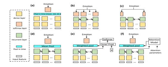
**Fig. 1**. Architectures for applying DNN/RNN for SER. (a) Learning LLDs using fixed temporal aggregation. (b) frame-wise training. (c) final-frame (many-to-one) training. (d) Mean-pooling in time. (e) Weighted pooling with logistic regression attention model. (f) general attention model.
