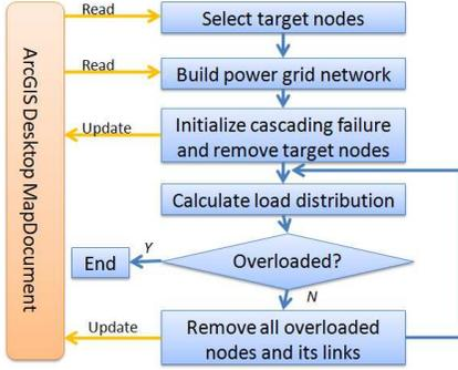
Fig. 1. The flowchart of the visualization platform.
