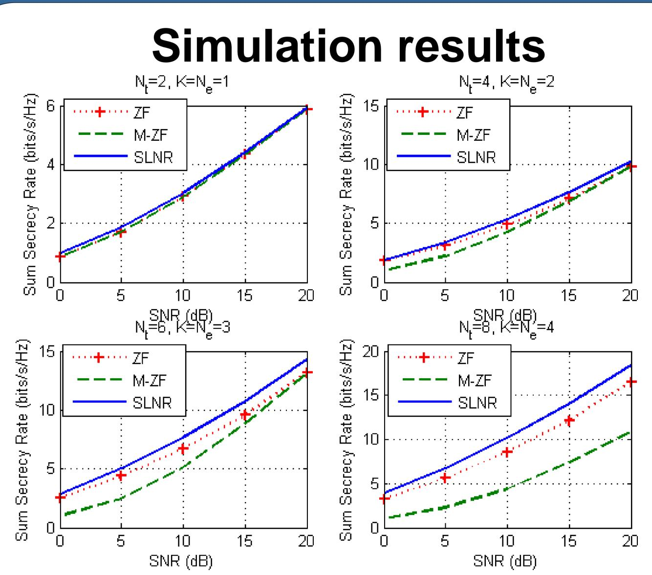
Fig.2. Achievable SSRs of the proposed beamforming algorithms. • "SLNR" has the best SSR performance, "ZF" is the second, while "M-ZF" is the worst; SSR performance gaps Of ♦the three these algorithms increase with K.
