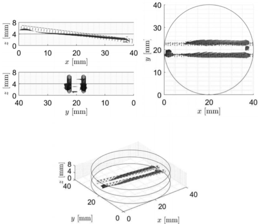
**Figure:** Model based reconstruction via ADMM and Stolt's f-k migration.
