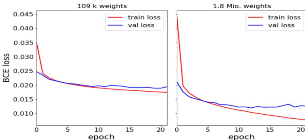
**Figure:** The loss curves of the proposed u-net variants.
