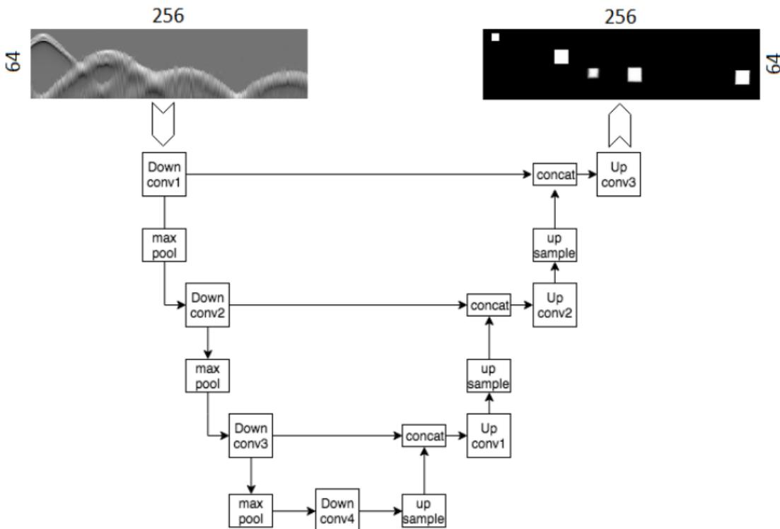
**Figure:** Architecture of the compact u-net.
