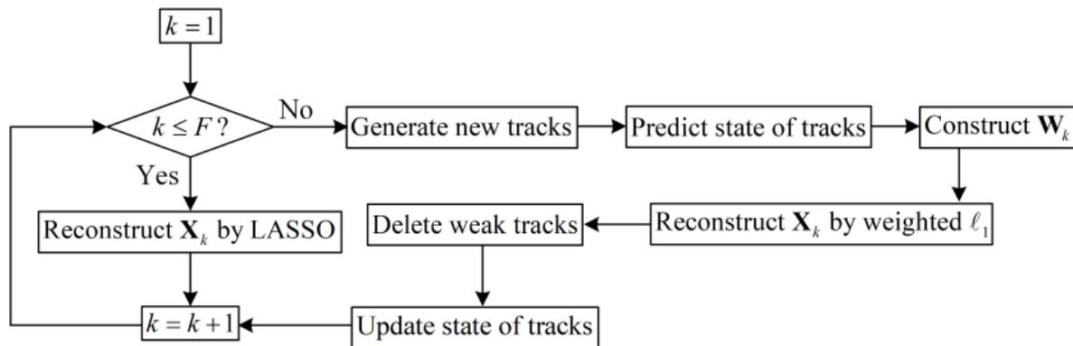
图: Flow diagram of WL1NM-TBD.
