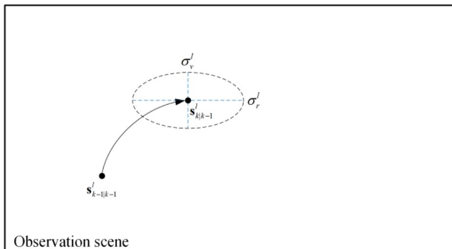
图: Formulating likelihood matrix  $\mathbf{J}$  with the prediction of Kalman filter.
