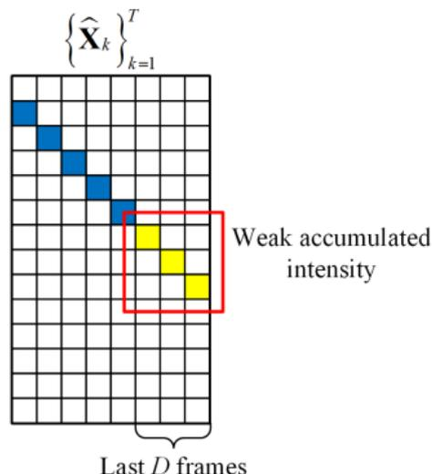
图: An example of deleting old tracks.
