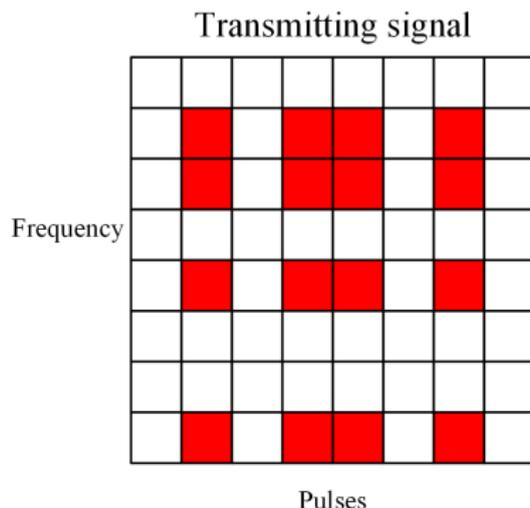
图: An example of the sub-Nyquist transmitting waveform in one CPI where  $P = N = 8$ ,  $\Psi = 2, 4, 5, 7$  and  $\Phi = 2, 3, 5, 8$ .
