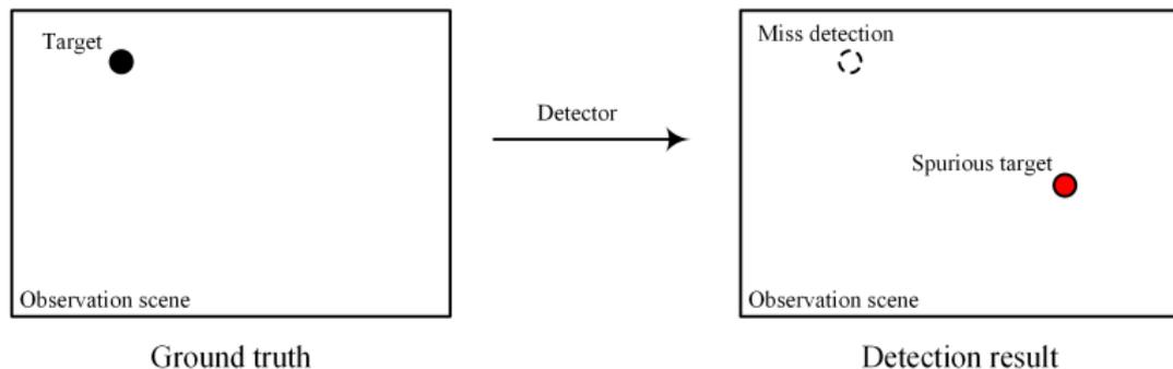
图: An example of miss detection and spurious target.
