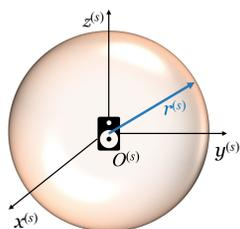
Figure 2: Measurement setup. The loudspeaker DIRs are measured at sampling points on the light red spherical surface of radius  $r^{(s)}$ .
