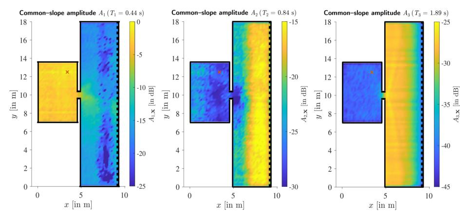
The late reverberation anisotropy becomes evident when beamforming into different directions and plotting the corresponding common-slope amplitudes.
