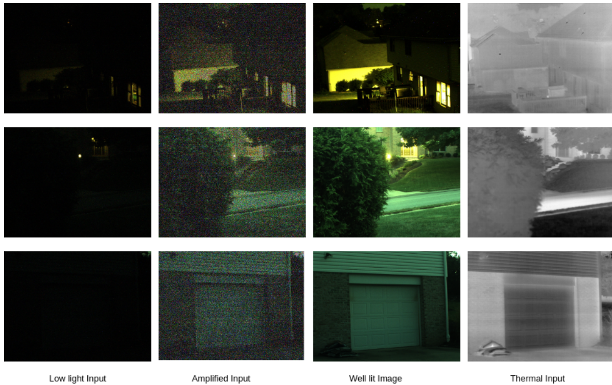
Fig. 2. The figure shows noise in our real-world V-TIEE dataset, showing low-light input, amplified input, well-lit, and corresponding thermal images. Amplified images, enhanced by a factor of 10, highlight the noise in low-light images.
