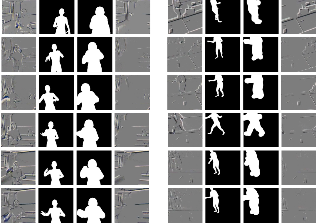
Fig. 1: Synthetic Dataset and Motion Segmentation Results. From left to right: the input voxel grid, the mask generated using the ground truth pose, the dilated mask, and the output voxel grid of the Motion Segmentation Module.
