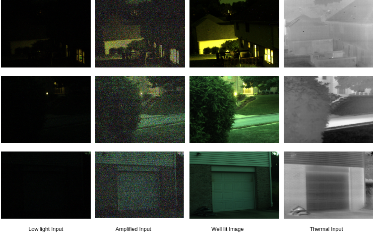
Fig. 10. The figure shows noise in our real-world V-TIEE dataset, showing low-light input, amplified input, well-lit, and corresponding thermal images. Amplified images, enhanced by a factor of 10, highlight the noise in low-light images.
