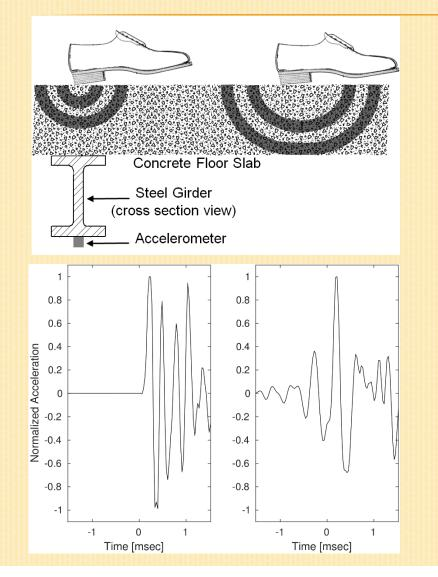
Footsteps directly above a girder-mounted sensor have a clear wave arrival (lower left), but those that travel laterally many meters undergo dispersion, reflections, etc. producing the complicated arrival wave (lower right)
