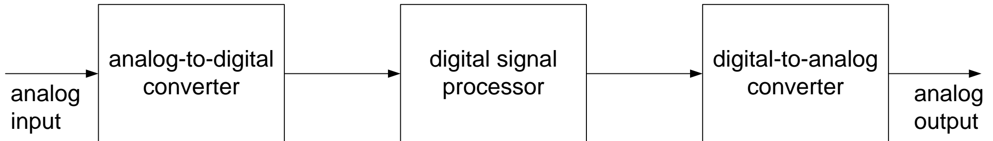
Fig.1.6: Digital processing of analog signal
