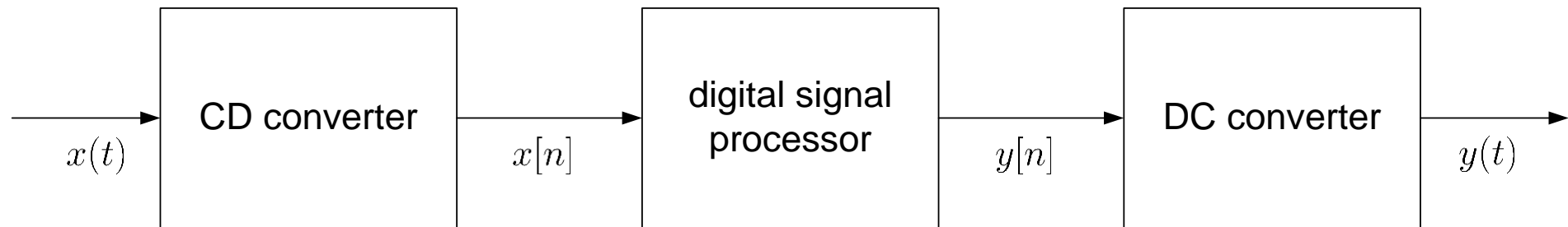
Fig.4.8: Ideal digital processing of analog signal
