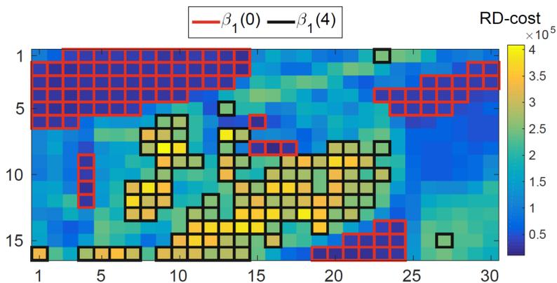
□ Relative RD-cost increase per CTU under constraint of the first frame of BQTerrace(1080p)
