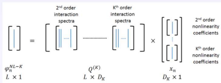
Proposed residual component model: RC-NL- $K$
