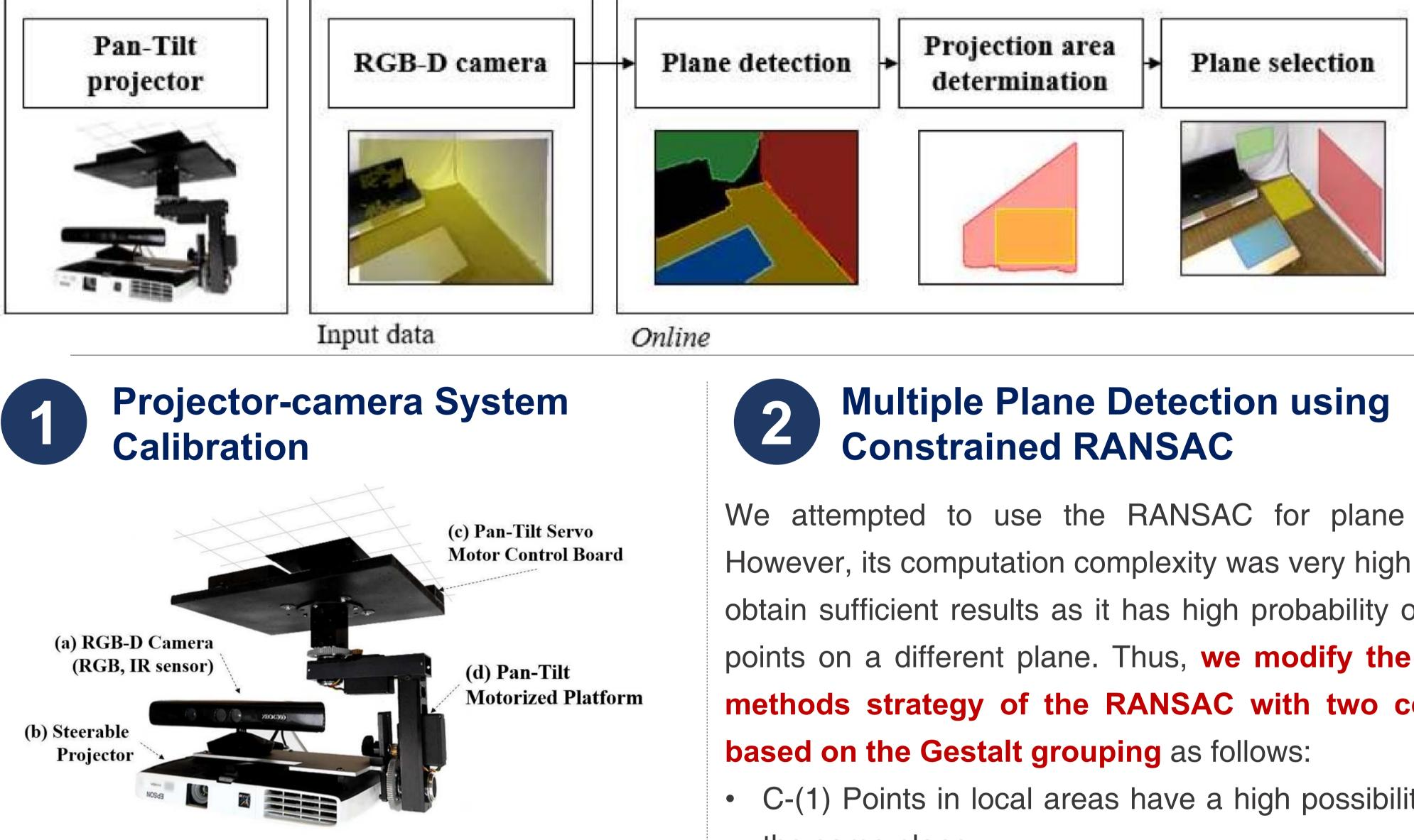
The 3D points in each device have different positions in each local coordinate system. Therefore, data from each sensor is **necessary to** be transformed into a common coordinate **system**. In our system, the relative position of the RGBD camera and projector is computed by using corner points on a checkerboard.
