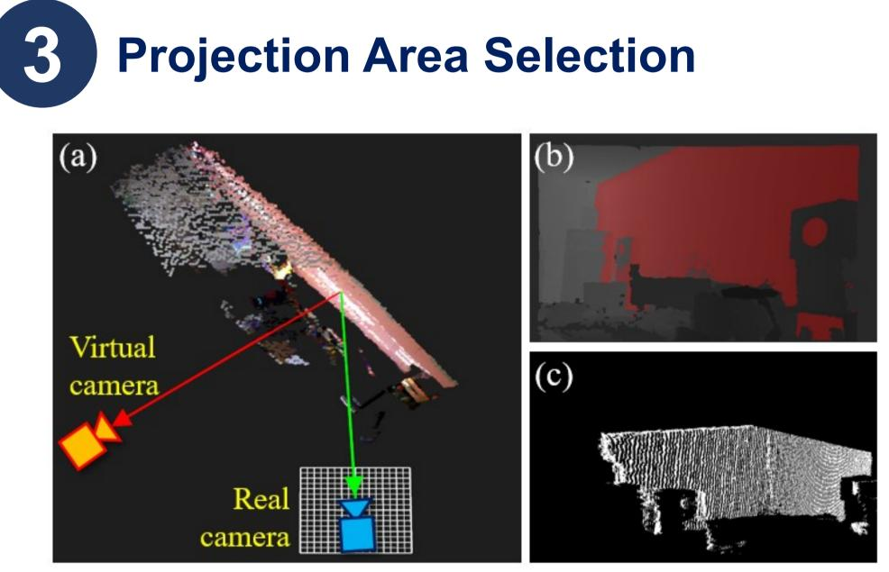
When the contents are projected on the planes directly, perspective distortion occurs from the viewpoint of the user. First, to correct this orientation difference, we first **place virtual cameras in front of**  $\Pi$  (a). Then, the point cloud of the plane is projected into the virtual camera. So, we can obtain an image of the front view (c) from the depth map (b). A rectangular area of maximum **size is selected** from the front view image.
