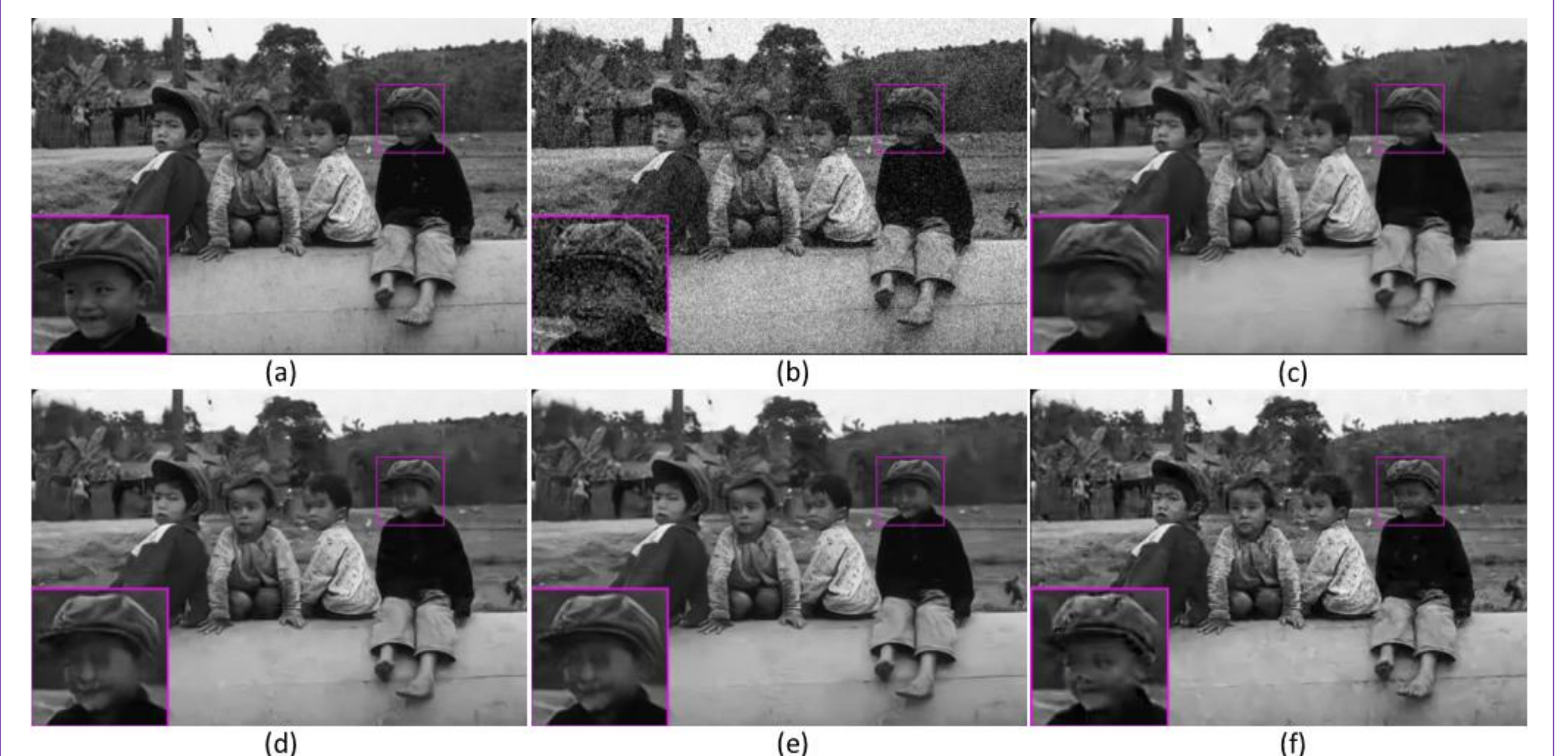
Fig.6 Denoising images of 15011 by different methods ( \sigma = 25 ). (a) Ground Truth; (b) Noisy image; (c) MLP (PSNR= 29.32dB); (d) TNRD (PSNR= 29.26dB); (e) Dn-CNN (PSNR= 29.46dB); (f) GSRC-EPLL (PSNR= 30.01dB ).
