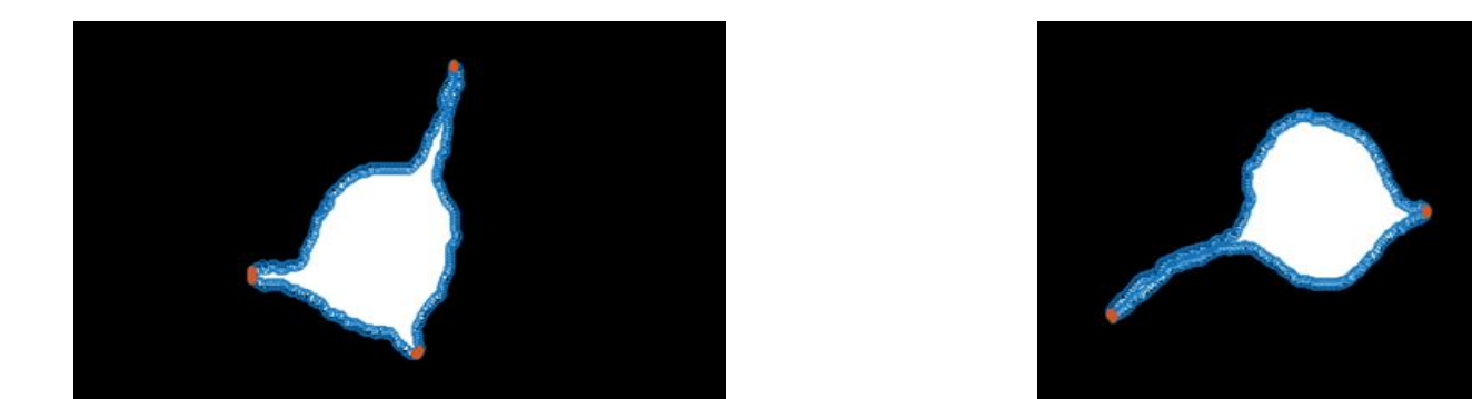
Tip detection result based on the distance to pre-learned Gaussian curve feature
