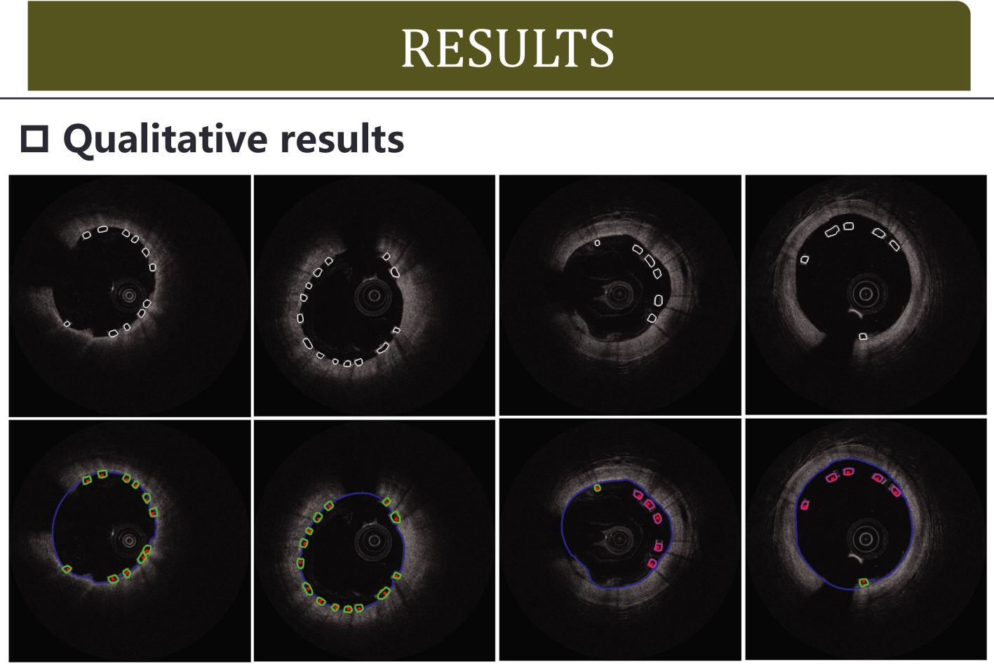
The first row is the images of ground truth marked by white curves. The second row is the segmentation results, where the green and purple curves represent apposed and malapposed struts respectively.
