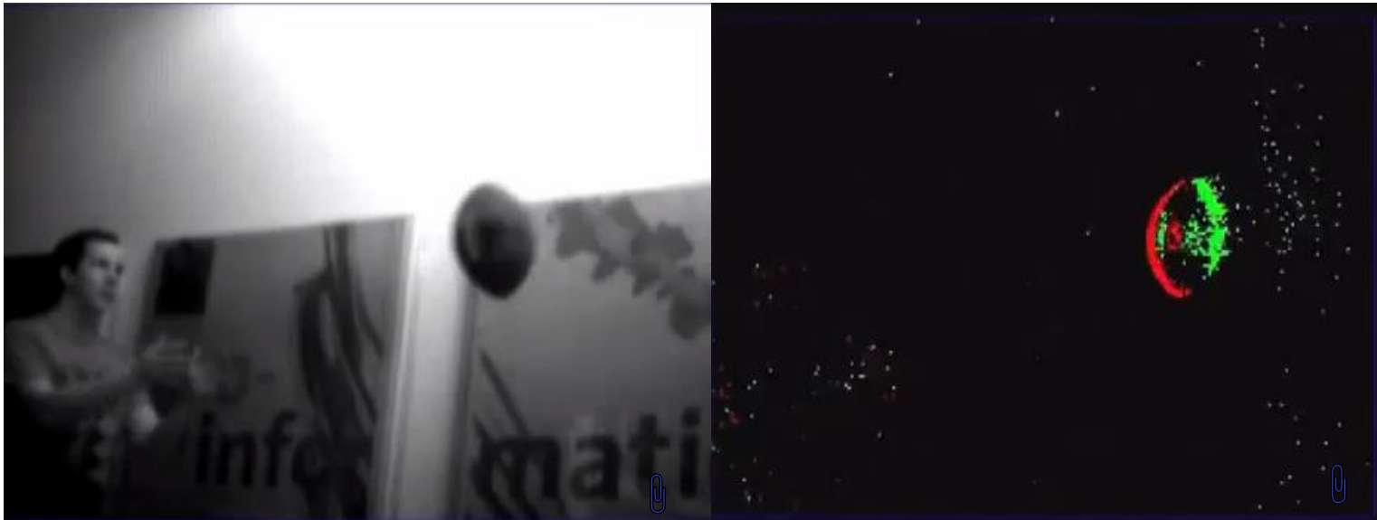
Fig.1. Conventional frames and Neuromorphic vision streams
