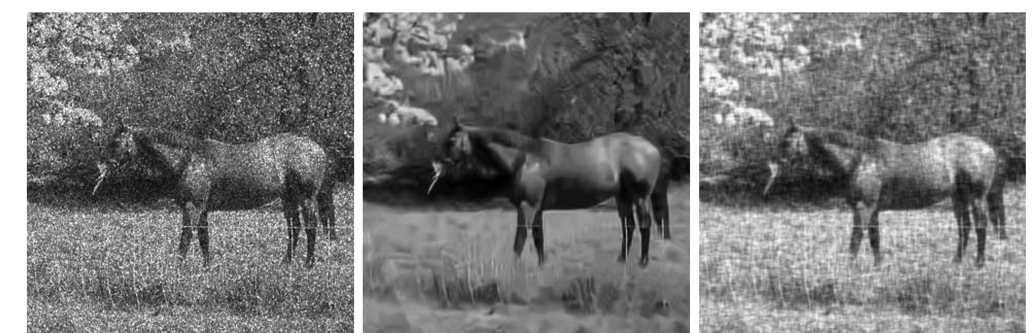
(d) MLE output. SNR= 8.87 dB PSNR= 13.28 dB SSIM= 0.37 (e) NI output. SNR= 15.78 dB PSNR= 20.19 dB SSIM= 0.41 (f) MMSE output. SNR= 15.6 dB PSNR= 20.01 dB SSIM= 0.51
