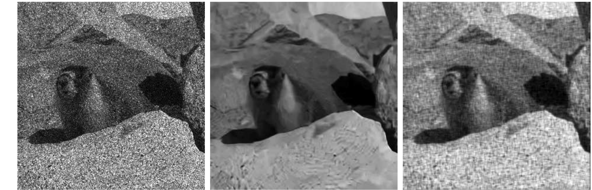
(a) MLE output. SNR= 8.29 dB PSNR= 16.34 dB SSIM= 0.37 (b) NI output. SNR= 15.58 dB PSNR= 23.63 dB SSIM= 0.55 (c) MMSE output. SNR= 15.51 dB PSNR= 23.56 dB SSIM= 0.60
