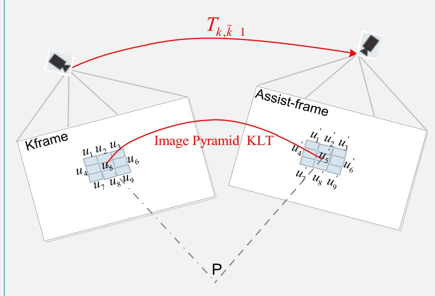
We build a fixed map to replace the incremental map used in previous works using the keyframe and the assist-frame only.
