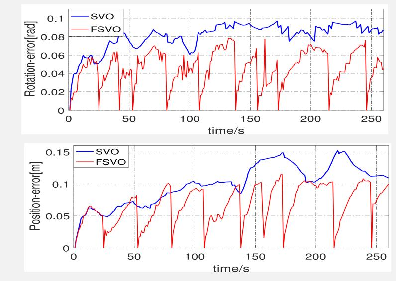
we run our algorithm on the KITTI dataset and the average position/rotation estimation error of SVO and FSVO is 0.0996m/0.0711rad and 0.0662m/0.0464rad, respectively.
