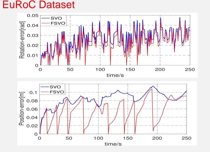
we run our algorithm on the EuRoC dataset and the average position/rotation estimation error of SVO and FSVO is 0.0783m/0.0262rad and 0.0554m/0.0223rad, respectively.
