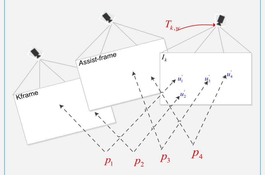
In this step, the camera pose and the structure (3D points) are optimized to minimize the reprojection error(motion-only BA problem).
