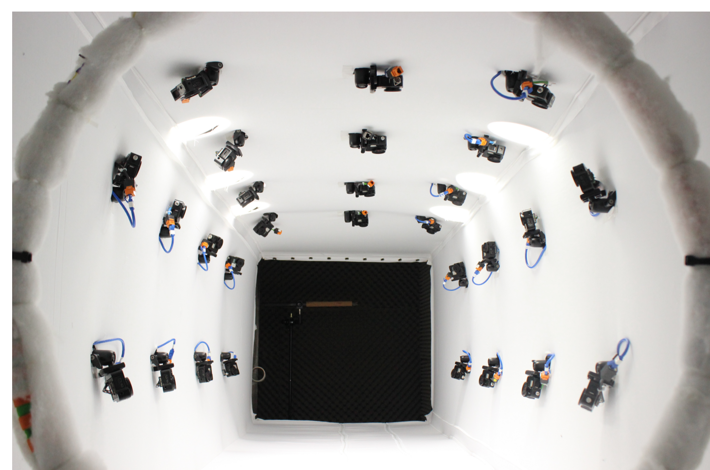
Figure 1: Flight Tunnel. 28 GoPro Hero 3+ Cameras running at 720p 120fps
