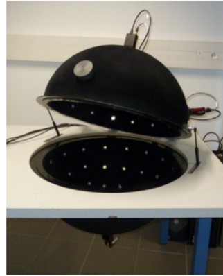
MeSurA Sphere ∅ 650mm 4 cameras 112 light sources
