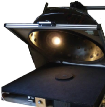
Dome v.1 ∅ 900mm 1 digital camera 96 light sources
