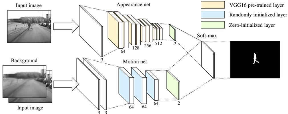
**Fig. 2.** Structure of proposed method. The proposed method consists of the appearance network (A-net) and the motion network (M-net). The A-net detects objects by focusing on appearance in image, and the M-net detects movement by comparing image and background image. The results of the two networks are combined to form a moving object detection result.
