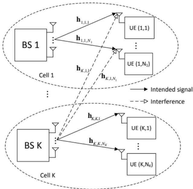
**Figure:** Downlink multiuser multicell interference scenario in a dense network consisting of  $K$  small cells and  $N_k$  single-antenna UEs in cell  $k$ .
