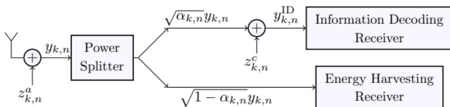
Figure: PS-based receiver structure at UE  $(k, n)$ .
