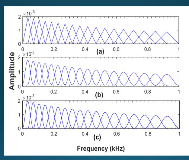
Magnitude normalized and linear warping scaled filterbank filters in kHz region
