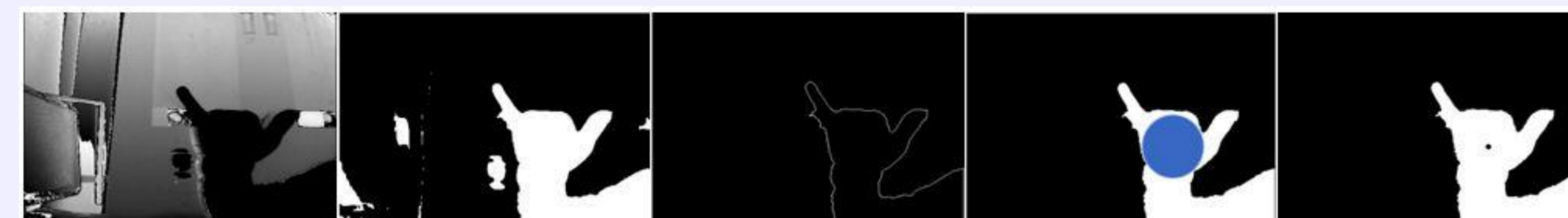
An example of seed selection on the depth map. Left to right: Depth map. Initial segmentation result by Otsu's method. Largest connected region. Variable-scale circle (blue). Seed selection result (seed: black point).
