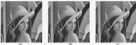
Fig. 3: Result on the noisy ( \sigma = 20 ) 512 \times 512 image Lena. (a) original, (b) noisy image, (c) denoised result.
