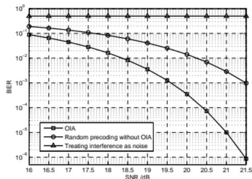
Figure: BER simulation results for different interference management schemes.
