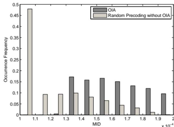
**Figure:** MID for pairwise channel parameters. As we test  $10^3$  pairwise channel parameters, the resulting MID distribution reveals that **the MID is significantly increased with OIA.**
