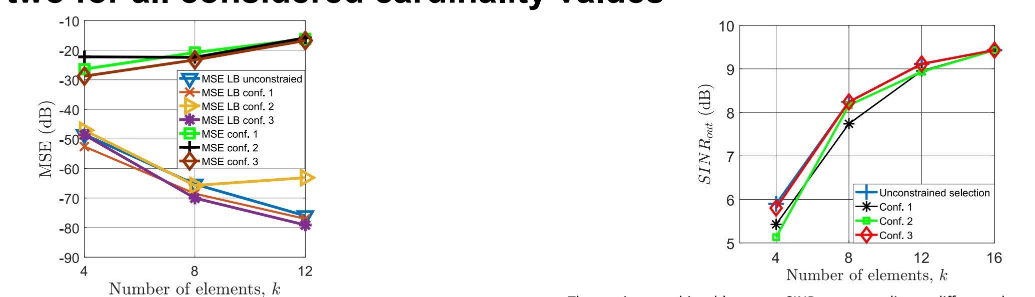
Top: MSE between clustered selection and unconstrained selection. Bottom: MSE between the optimum value obtained by exhaustive search and SDR. The maximum achievable output SINR corresponding to different cluster cardinalities for unconstrained spatial thinning and spatial thinning under different connectivity constraints
