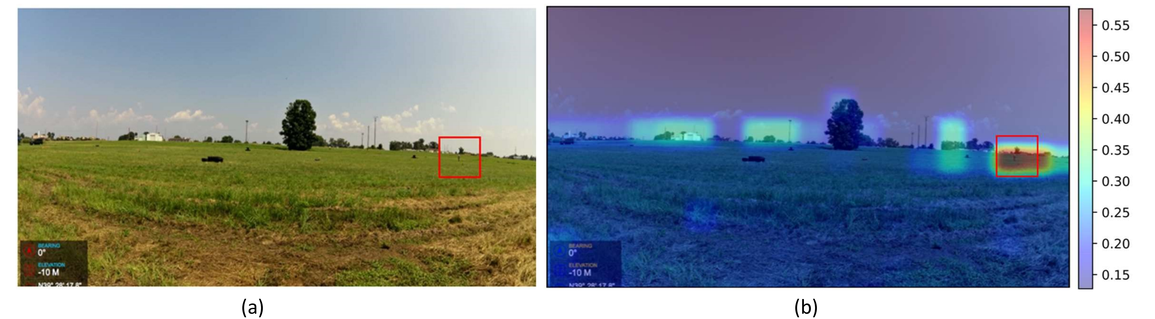
Detection result on a frame captured from a different angle shows robustness of the proposed algorithm: (a): Original video frame, (b): Detection Probability when network was trained using proposed Cross-Modal distillation. Red box marks true location of target
