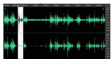
Fig. 7 Waveforms. SBRES+SBNR+NLEC reduces ~40 dB echo (top = Off, bottom = On)
