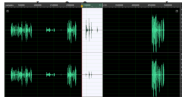
Fig. 5 Waveforms. SBRES reduces ~11.64 dB echo (top = Off, bottom = On)
