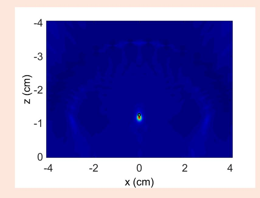
MIMO radar imaging to detect the tumor location: (a) Conventional MIMO radar where the clutter is subtracted from the complete FDTD results with tumor. Symbol "o" represents the centroid of the tumor and \* represent the peak of the image; and (b) Coherent FFTR-MUSIC with the TR clutter suppression method.
