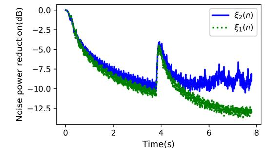
Figure 4: Noise cancellation simulation: The noise power reductions at error sensor one  $(0.09, 2.0, 0.0)$  m achieved by the proposed system  $\xi_1(n)$ , and by the conventional system  $\xi_2(n)$ .
