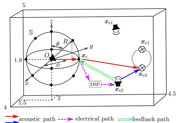
Figure 1: A broadband ANC system in a reverberant room.
