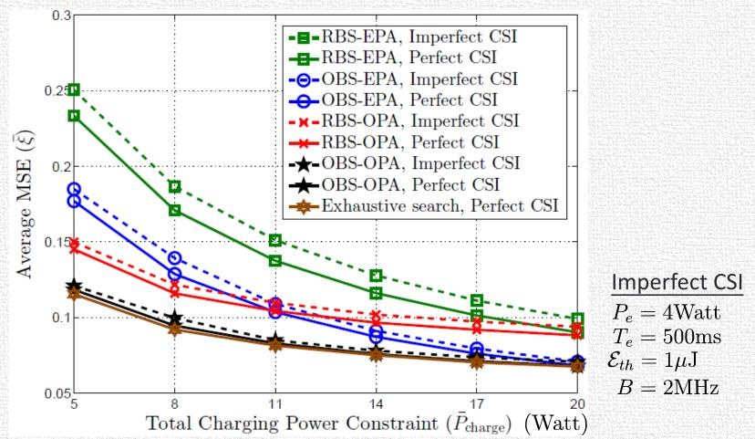
**OBS-OPA** : Optimized Beam Selection and Optimized Power Allocation **OBS-EPA** : Optimized Beam Selection but Equal Power Allocation **RBS-OPA** : Random Beam Selection but Optimized Power Allocation **RBS-EPA** : Random Beam Selection and Equal Power Allocation
