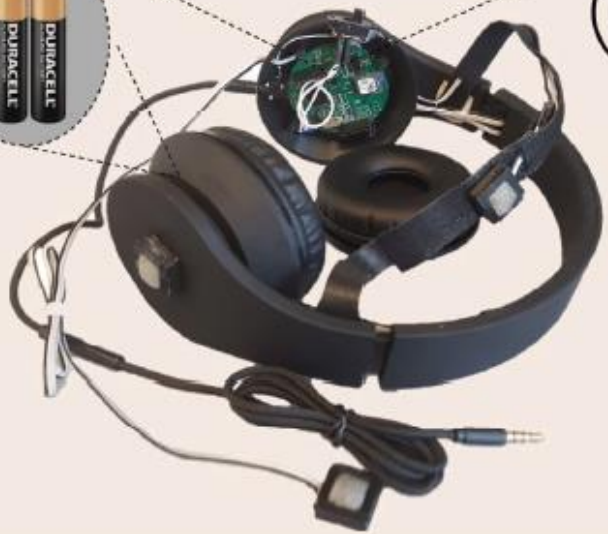
FIGURE 4. The prototype intelligent pedestrian safety headset and connected smartphone.
