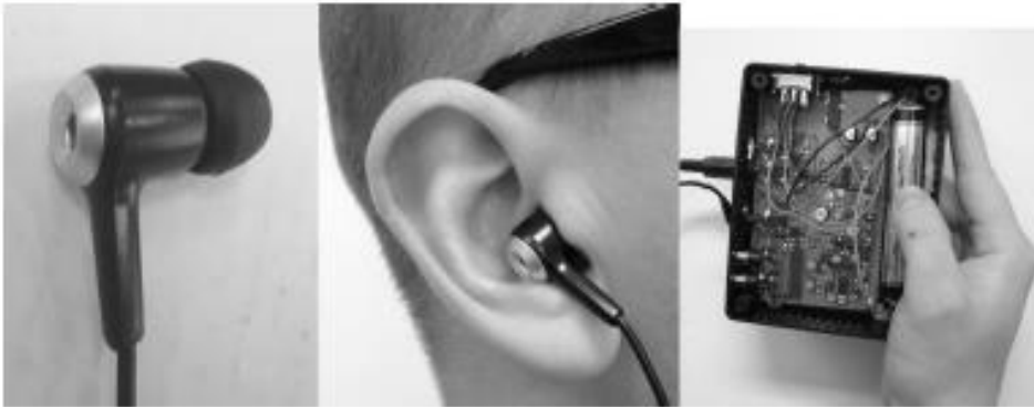
Left and middle: ARA headset (Philips SHN2500) Right: Prototype ARA mixer
