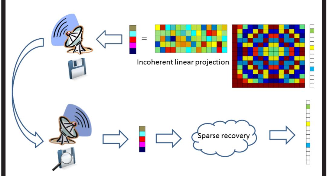
Compressed Sensing allows for compression of sparse signals before transmission/storage and reconstruction when required.
