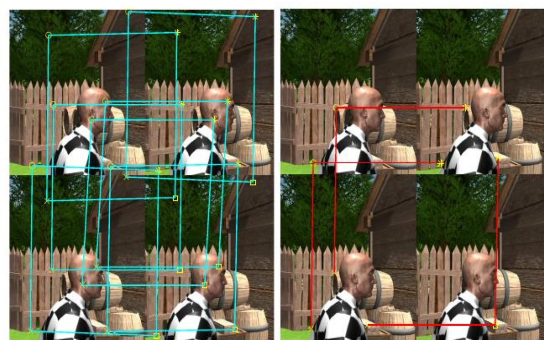
Fig. 1: Constructed commonly-identified feature set: The control points only connected by red line in vertical or horizontal direction will be rejected. Only the control points connected by yellow line in both of vertical or horizontal direction will be selected for Commonly-identified feature set.
