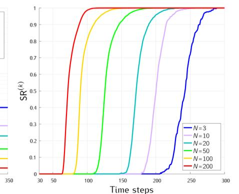
Left: Averaged PEB as a function of  $N$  with  $d_{\text{hop}} = 20$  m and  $h_{\text{max}} = 1$ ; Right: Success rate vs.  $N$  with  $d_{\text{hop}} = 20$  m,  $h_{\text{max}} = 1$  and  $\xi^* = 0.5$  m
