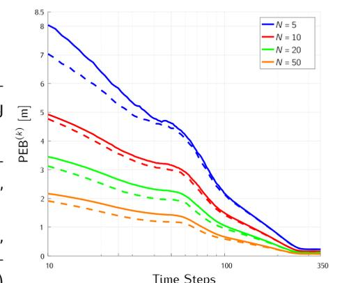
Averaged PEB vs.  $h_{\text{max}}$  with  $d_{\text{hop}} = 20$ . Dashed lines refer to the case  $h_{\text{max}} = 3$  while continuous lines to  $h_{\text{max}} = 1$
