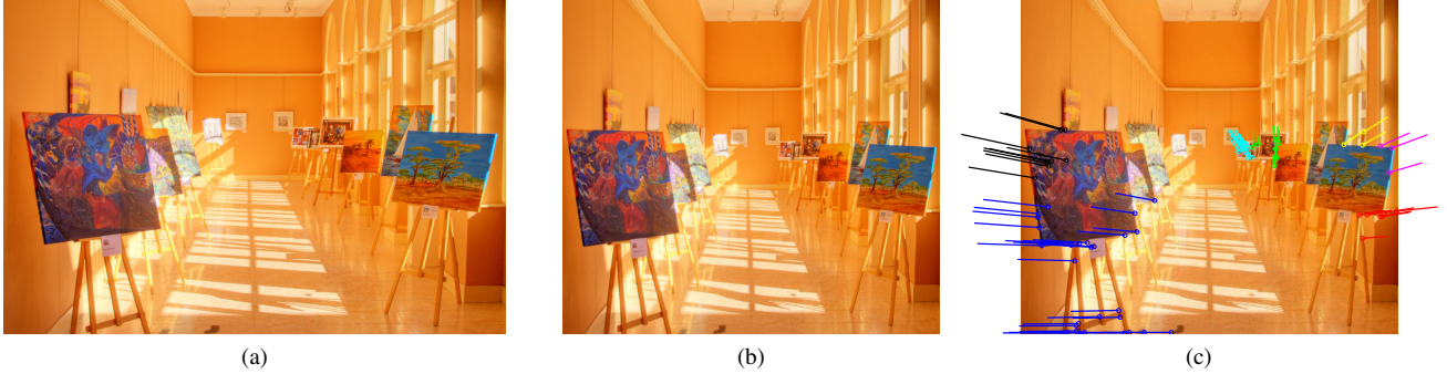
Fig. 6: Illustration for spatial clustering: (a) original image, (b) its resized image by a retargeting algorithm called Streaming Video [18], (c) resized image overlaid with spatial clustered displacement vectors
