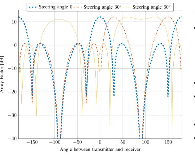
UPA beamforming patterns (using 3GPP approach) • Array factor for each device
