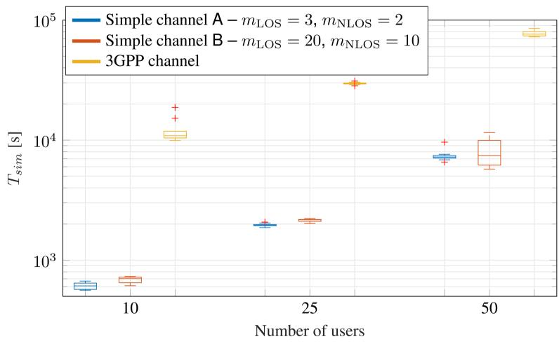
Simulation execution time: 3GPP takes 10 times longer Higher traffic also translates into high execution time A factor of 5 in the number of users is a factor > 10 in the execution time
