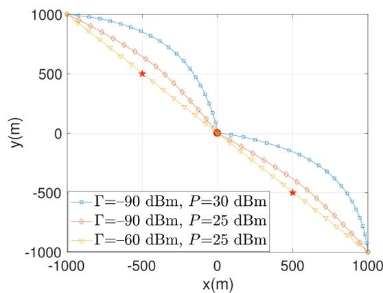
(a) UAV trajectories projected onto the ground (horizontal) plane by the proposed design with joint UAV trajectory and power optimization. The red stars represent the locations of the two ground PRs, respectively, and the red circle denotes the location of the ground SR.
