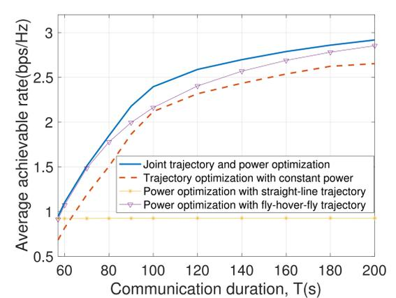
(b) The average achievable rate of the cognitive UAV communication versus the communication duration  $T$ .
