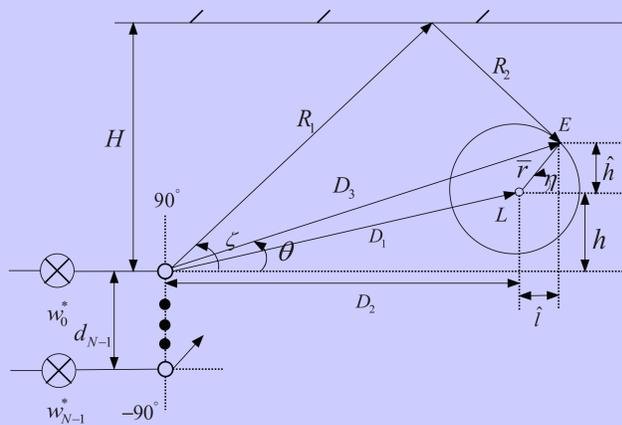
Figure 1: Multi-path signal transmission to the desired receiver  $L$  and eavesdroppers  $E$
