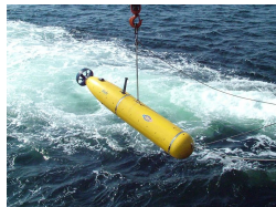
(c) Autonomous underwater vehicle (AUV) for search and rescue, security, and scientific uses 3
