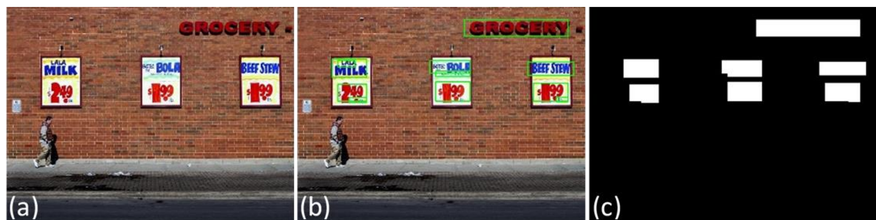
Result of text detection. (a) Input image, (b) Text detection (green bounding-boxes), and (c) Binary text masks.
