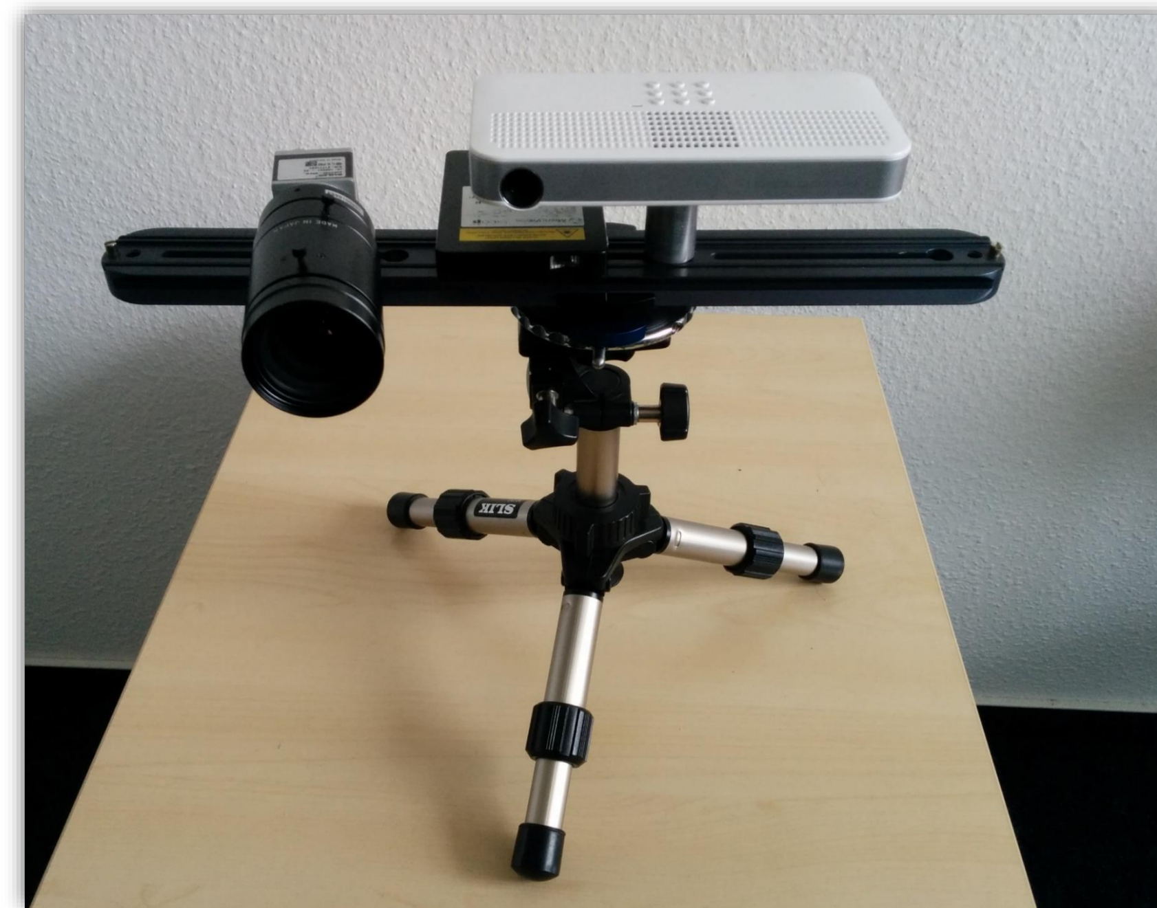
Intrinsically and extrinsically calibrated projector-camera system.
