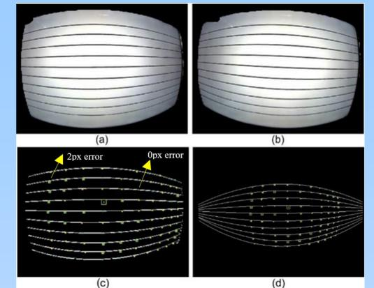
Fig 3: (a) left (b) right *e-curve* images for cam. setup 1; (c) *e-curves* extracted from (a); (d) curve fitting result of (c)
