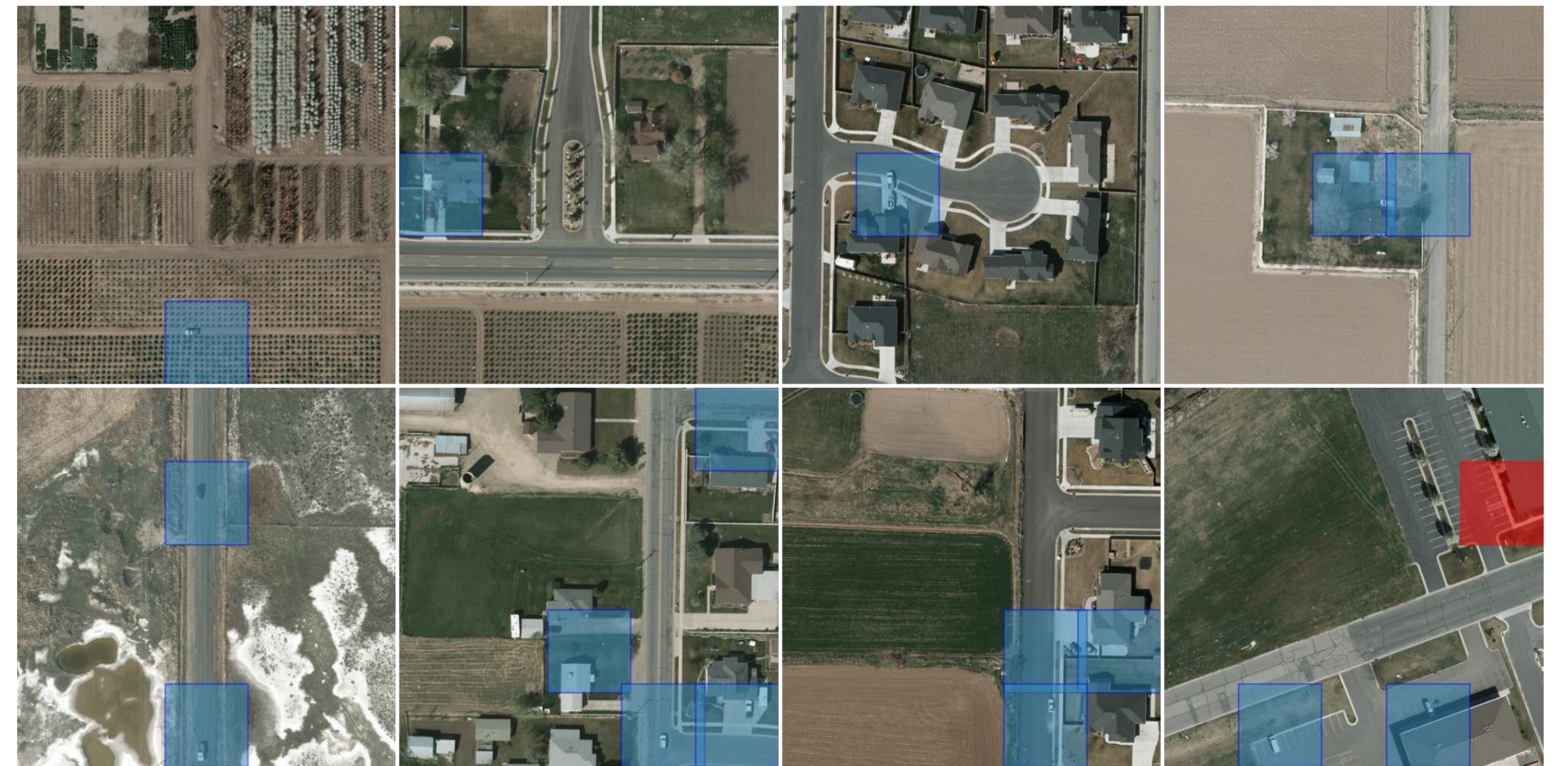
Fig. 3: Qualitative examples of the SAR module exhibit that the search area is clearly reduced. Highlighted regions are considered for detection. Regions labeled in blue contain at least one vehicle whereas the region labeled in red contains no vehicle.
