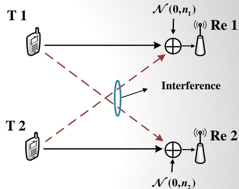
Two-user Gaussian interference channel
