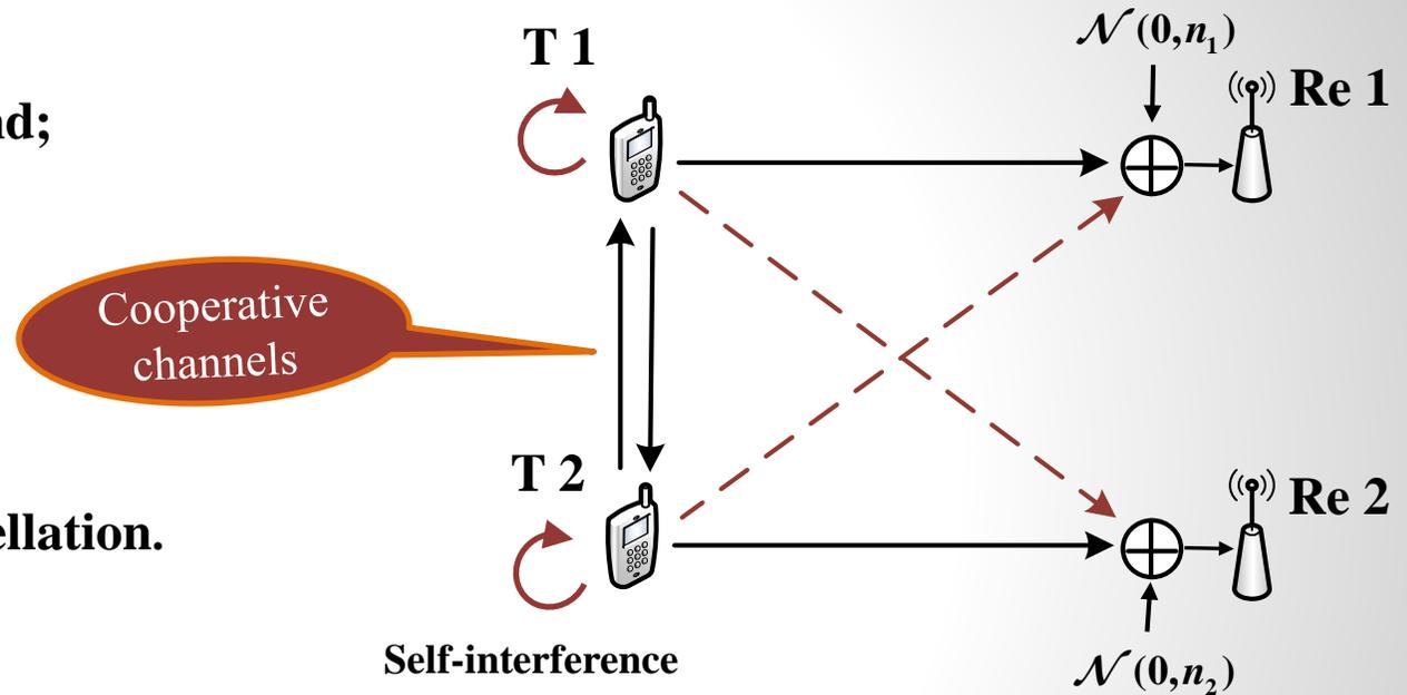
Interference channel with transmitter cooperations
